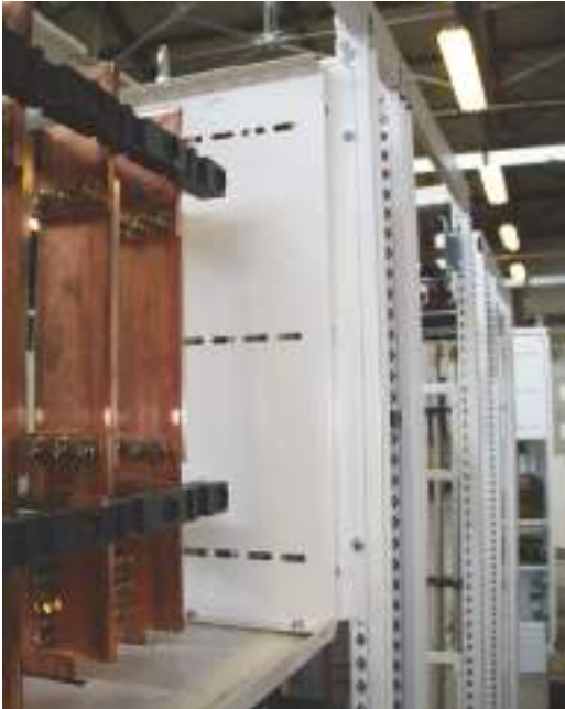
Dismountable vertical busbars.
